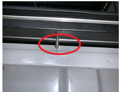
Place the assembled sliding nut kit on the track and slide to proper place (A04 A01)
