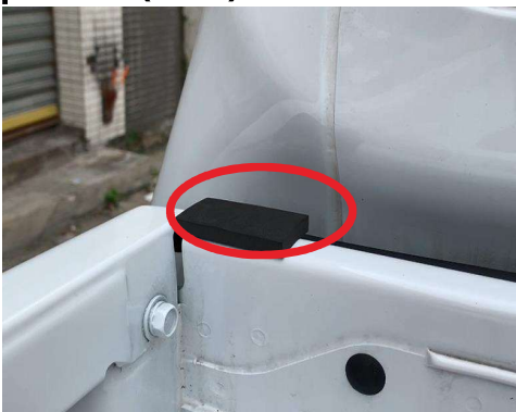
If not horizontal, then adjust the lower side bar with A24 Track Angle Shim or A03 Foaming Adhesive Tape
